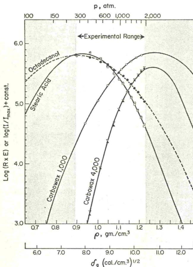
Figure 3. Detector response ( $R \times E$ ) and relative solubility ( $X_2/X_{2,max}$ ) at  $40^\circ$  as a function of CO<sub>2</sub> density,  $\rho$ , solubility parameter,  $\delta$ , and pressure,  $P$ .
